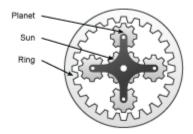
In fuel economy and powertrain studies, you can use the Planetary Gear block as a power-split device by coupling it to common driveline elements such as transmissions, engines, clutches, and differentials.
