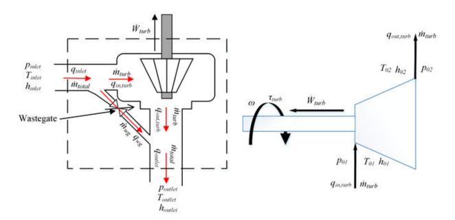
The Turbine block implements equations to model the performance, wastegate flow, and combined flow.
