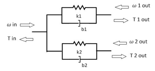
$$T_{in} = -(\omega_{in} - \omega_{1out})b_1 - (\omega_{in} - \omega_{2out})b_2 - \theta_1 k_1 - \theta_2 k_2$$
