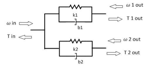
$$\begin{split} T_{out} &= (-\omega_{out} + \omega_{1in})b_1 + (-\omega_{out} + \omega_{2in})b_2 + \theta_1k_1 + \theta_2k_2 \\ T_{1out} &= (\omega_{out} - \omega_{1in})b_1 - \theta_1k_1 \\ T_{2out} &= (\omega_{out} - \omega_{2in})b_2 - \theta_2k_2 \\ \dot{\theta}_1 &= (\omega_{1in} - \omega_{out}) \\ \dot{\theta}_2 &= (\omega_{2in} - \omega_{out}) \end{split}$$
