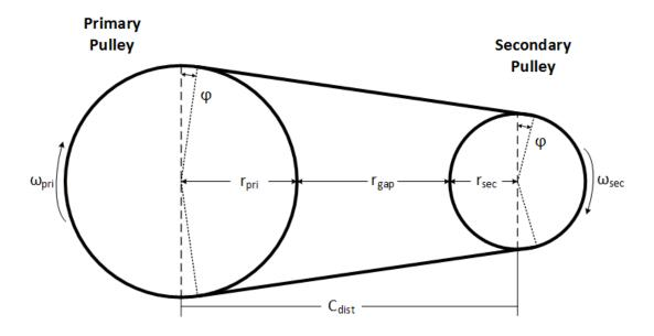
$$C_{dist} = rp_{max} + r_{gap} + r_{sec\ max}$$
