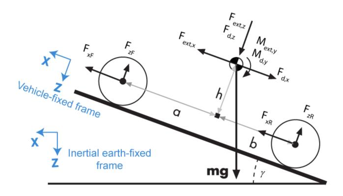
The Vehicle Body 1DOF Longitudinal block implements these equations.
