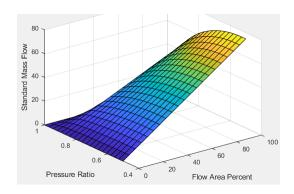
EGR valve standard flow pressure ratio breakpoints, f\_egr\_stdflow\_pr\_bpt —  $\mbox{\bf Breakpoints}$
