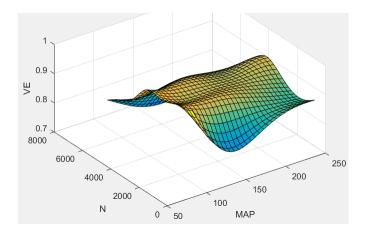
**Speed-density intake manifold pressure breakpoints, f\_nv\_prs\_bpt — Breakpoints** vector
