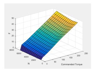
The main start-of-injection (SOI) timing lookup table is a function of commanded fuel mass and engine speed
